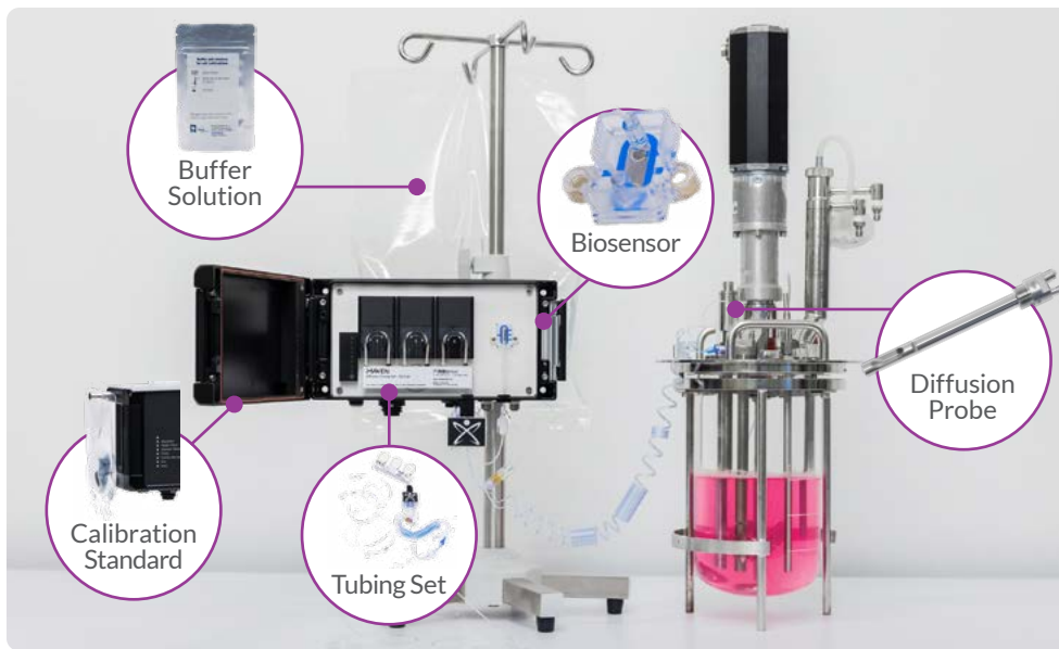
Figure 1. MAVEN components and connection to a 2L, single-walled bioreactor from Sartorius
